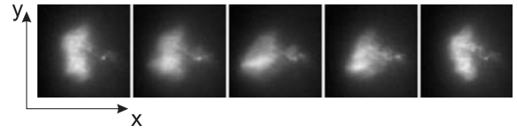
Fig. 1. Sequence of snapshots showing the time evolution of the unstable atomic cloud. Snapshots are presented in the chronological order, each one being separated by 40 ms. This sequence corresponds to the fast stage of a C_P cycle (see Sect. 3).
