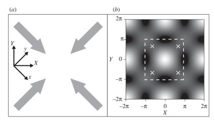
Figure 1. (a) Layout of the laser beams. (b) Spatial distribution of the intensity in the (X, Y) space. Black corresponds to the minimum value (zero intensity), while white corresponds to the maximum. The dotted square delimits the elementary mesh of the lattice, and the white crosses are the saddle points.
