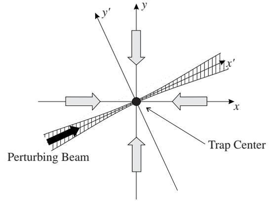
**Fig. 1.** Experimental set-up. The PB is contained in the plane formed by the  $x$  and  $y$ -axes of the MOT, and makes an angle  $\theta$  with the  $x$ -axis. The  $z$ -axis is perpendicular to the plane of the figure.
